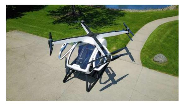
Surefly is a two-seats personal helicopter with eight independent motors each driving a single carbon fiber monopropeller, a battery pack and a ballistic parachute in case of emergency landing. The company's motto is to bring an affordable and easy-to-pilot flying experience to its customers.
