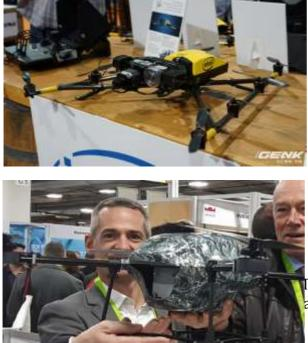
The **Falcon 8+** drone is developed by **Intel** to inspect industrial sites by providing a stable flight. The drone provides real-time different data by 3D reconstruction with millimetre accuracy. Its goal is to detect industrial flaws.
