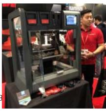
The US Company **Airwolf** was presenting **EVO**, a <sub>3</sub>D printer for manufacturers. The main assets are its large size, its multimaterial uses and its resistance to high temperatures. According to its leaders, it is faster, more powerful and more accurate than most <sub>3</sub>D printers.
