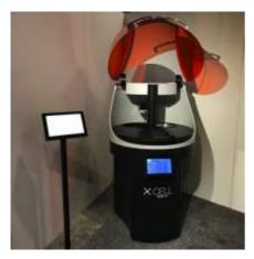
The **XCELL 3D** printer developed by the Italian company DWS uses a 3D stereolithographic printing system. **DWS** integrates a washing and drying system in this 3D printer. Thus, there is no need for any intervention while submitting a file. After printing, the build plate elevates and moves objects into a second chamber for washing. In the next step, the plate dips the objects into a third chamber where they are cured to remove any residue.
