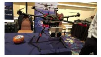
**Fotem** develops a drone that sends nets and recovers drones that venture on its territory day and night, in rainy weather or good weather. A product to secure sensitive industrial sites from intrusions.
