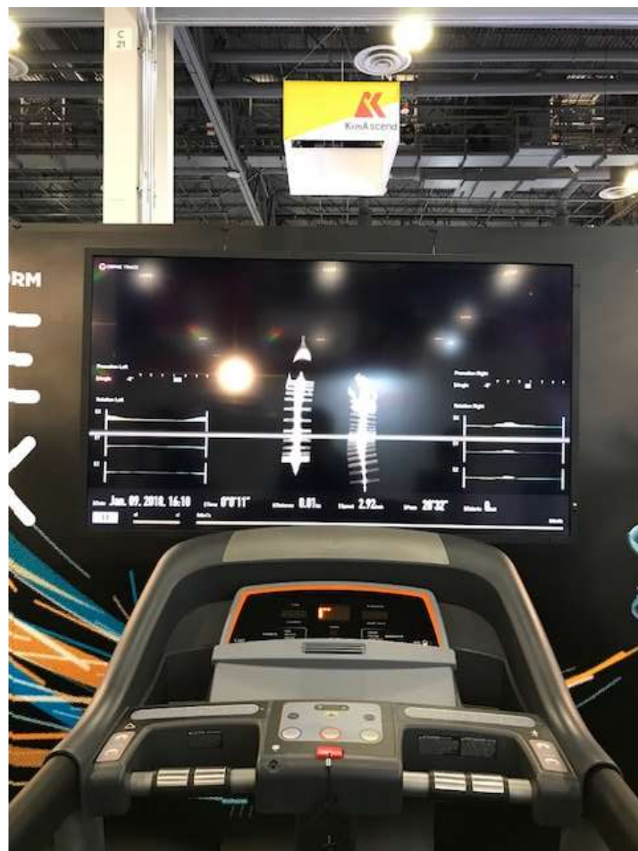
Here is Orphe Track treadmill, which analyses the runner's stride on the screen
