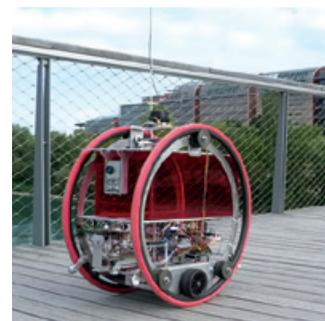
TwinswHeel is an autonomous parcel delivery droid. We design and manufacture the droids that will contribute to the future of urban logistic. The first step is to focus on enclosed sites such as large industrial sites and, shortly after, cities with e-commerce and convenience stores. Our droid is based on the autonomous vehicle in order to succeed in the self-sufficient goods delivery business. TwinswHeel is a smart, flexible and efficient droid for all year round delivery 24/7.
