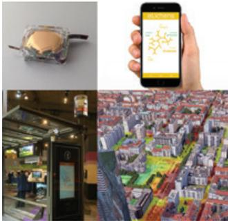
elichens platform delivers Air Quality high resolution digital mapping at an optimized cost and a fast time to deploy. Our unique platform is powered by best in class gas dispersion model & in house cost effective sensors. The Air Quality data becomes now relevant and it allows personalized services. elichens solutions come with a disruptive and patented Multi-gas (CO2, CH4 ...) optical MEMS sensors based on NDIR which address both industrial & consumer electronics markets.
