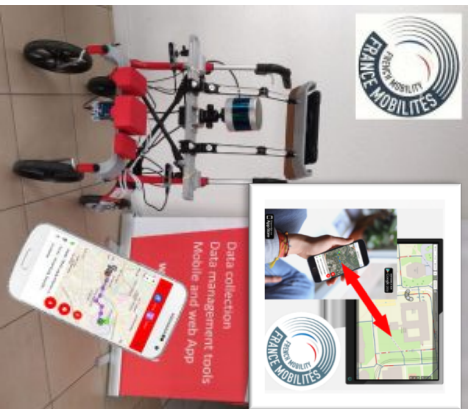
Real-Time 3D scanning system for Accessibility diagnosis of cities
