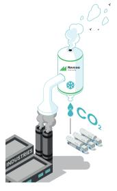
Revcoo develops a CO2 capture process (PCC) for industrial facilities. Its technology is based on a patented combination of antisublimation and continuous carbon separation, the CarbonCloud®. This clean and sober process allows all emitters to capture their CO2 emissions.
