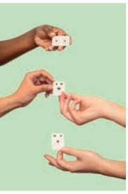
BeFC creates electricity with papers and enzymes for portable electronics. Along with this disruptive sustainable thin energy source, BeFC provide ecofriendly ultra-low power electronic platforms. These platforms are thin, flexible and can combine a range of sensors, microcontrollers. user interactions and wireless modules including NFC, BLE, LoRaWAN or Sigfox to build bespoke solutions for our clients in markets including medical, healthcare, logistics & waste management.
