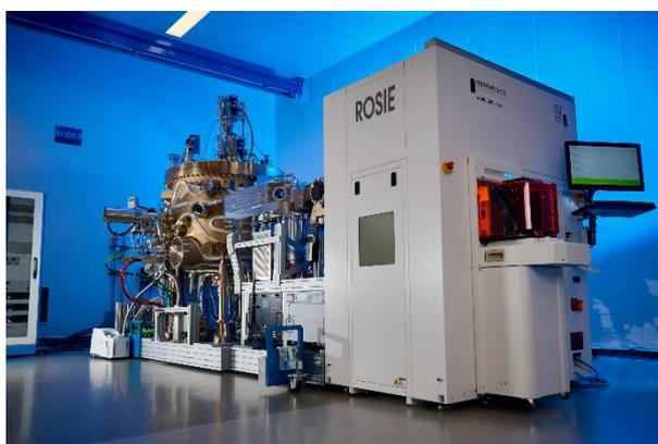
This order represents a key milestone in the development of ROSIE, RIBER's latest innovation. Fully automated and compatible with 300 mm silicon wafers, ROSIE is designed for the growth of thin oxide layers, particularly barium titanate (BTO), a strategic material for the development of integrated electro-optic modulators.
